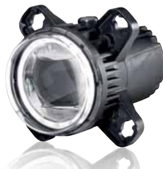
LED low beam headlamp L 4060 with daytime running/position light*
