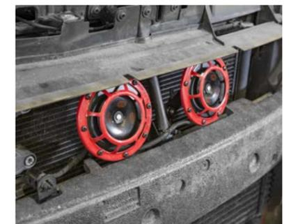
If the functional test is successful, the bumper cover can once again be mounted with all assembly parts, thus fully restoring the vehicle.
