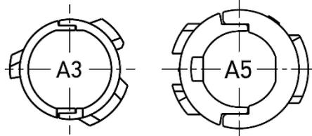
Information: In case you can't insert the HERO integration connector into the OE bulb sockets, cut off the tabs on the side. The connector will still grab the socket and will sit tight.
