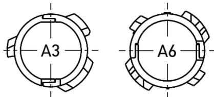
Information: In case you can't insert the HERO integration connector into the OE bulb sockets, cut off the tabs on the side. The connector will still grab the socket and will sit tight.
